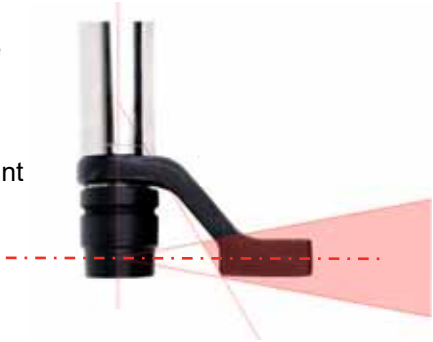
FIGURE 7 – Standard Length Socket Safe Reaction Window
